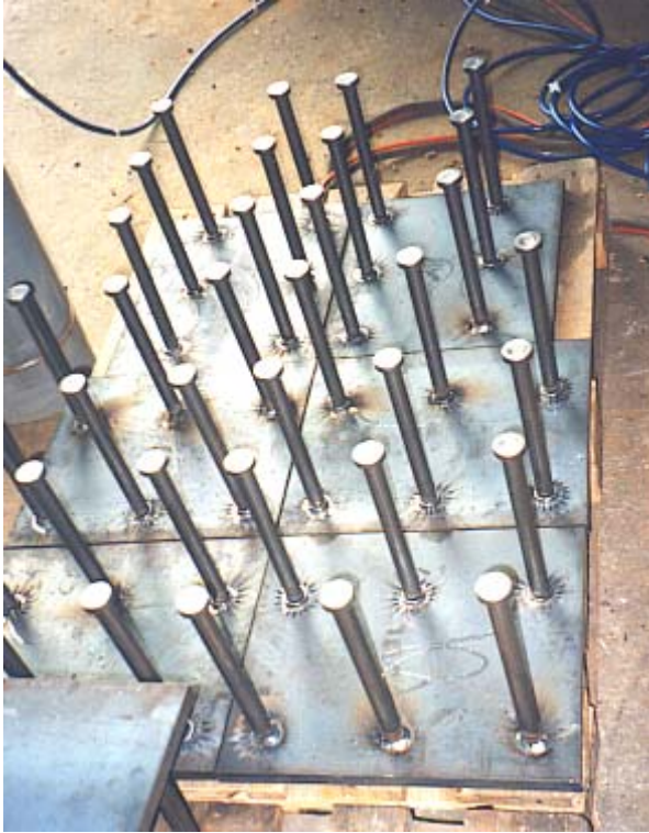
Figure 14: Anchor plates with welded-on KÖCO shear connectors in production
