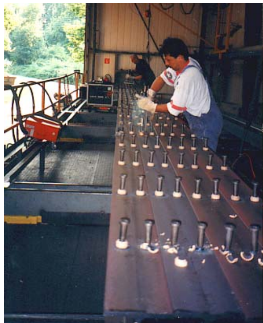
Figure 4: Stud welding in the mass production of composite beams
